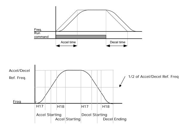
• Note that setting Frequency Ref. for Accel/decel (H70) is set to Max Freq and target freq is set below Max freq. the shape of S-curve may be distorted.
